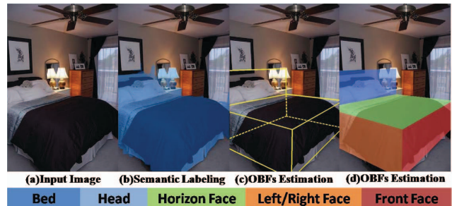
Figure 1. The motivation of our method. (a) The input image, (b) semantic labeling result, (c) and (d) are both the OBFs estimation results (in different visualization). In (c), yellow lines indicate the 3D structure lines aligned to the object. In (d), different color illustrates different faces of an object.
