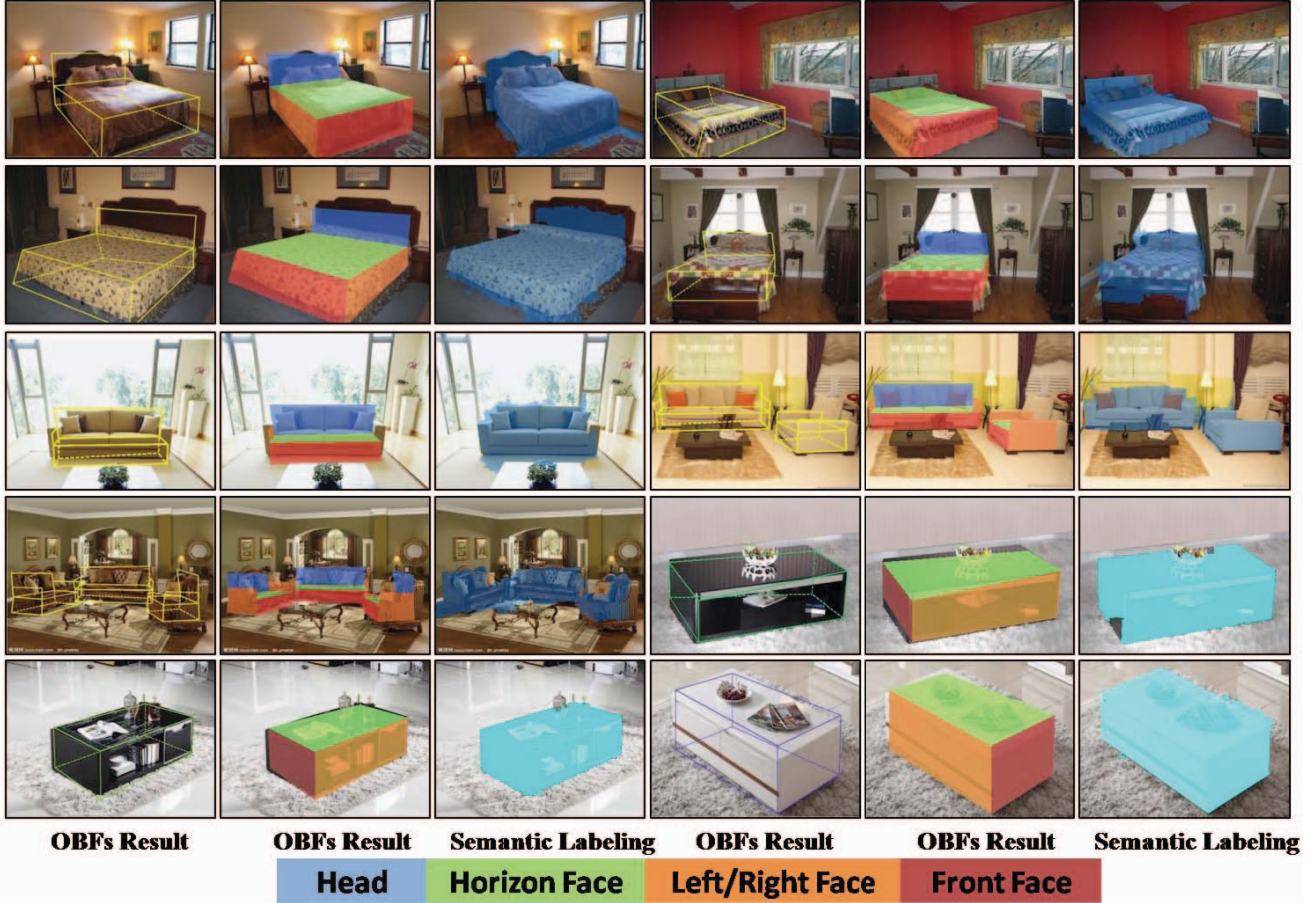
Figure 7. Our results of both bedroom and living room. Column 1 and 4 are the results of OBFs estimation, visualized in aligned object. Column 2 and 5 are also the results of OBFs estimation, which visualized in colored faces. Column 3 and 6 are the results of semantic labeling, where legend bar is shown below.
